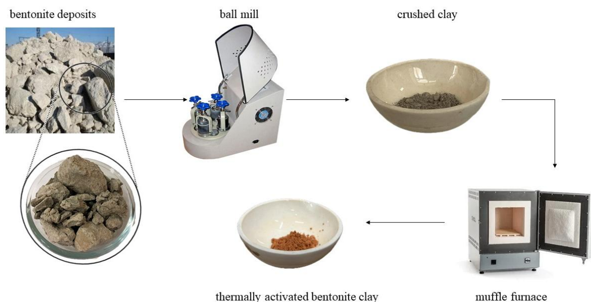
Figure 1 – Scheme of thermal modification of bentonite clays
